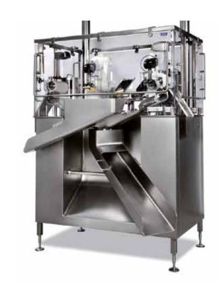
THE AUTOMATED PLASMA THAWING AND BAGS EMPTYING PROCESSES OFFER MAXIMUM SAFETY AS PLASMA IS NOT HANDLED BY THE OPERATOR WHILE THE BAGS ARE OPEN, THEREBY MINIMIZING POSSIBLE EXTERNAL CONTAMINATION AND ALSO REDUCING COSTS AND INCREASING PERFORMANCE.
