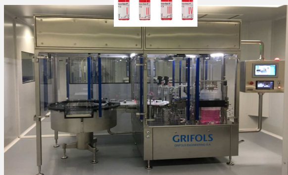
Automated red cells filling machine; Barcelona
